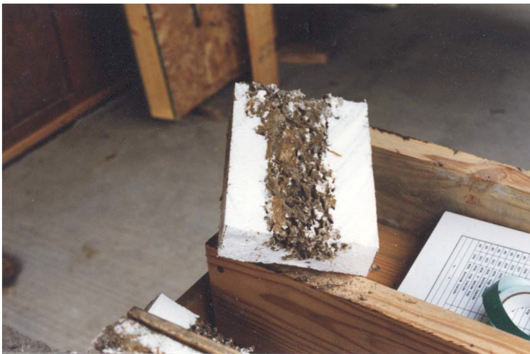
#45 TEST FIXTURE - Close-up shows nesting infestation of termites.
