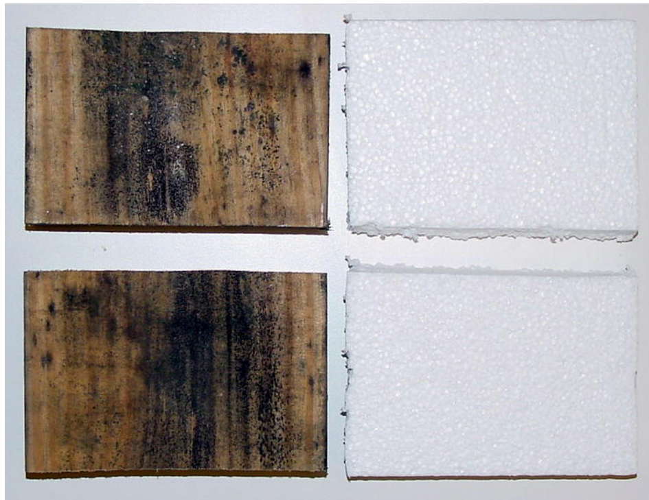
Southern Yellow Pine with Mold Growth
