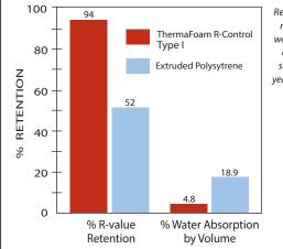
Retained thermal resistance and water absorption of insulations subjected to 15 years below grade exposure
