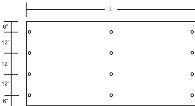
Connection patterns for two span condition
