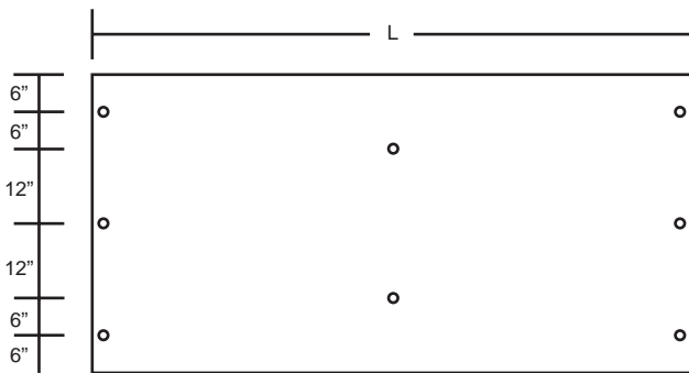
Connection patterns for two span condition
