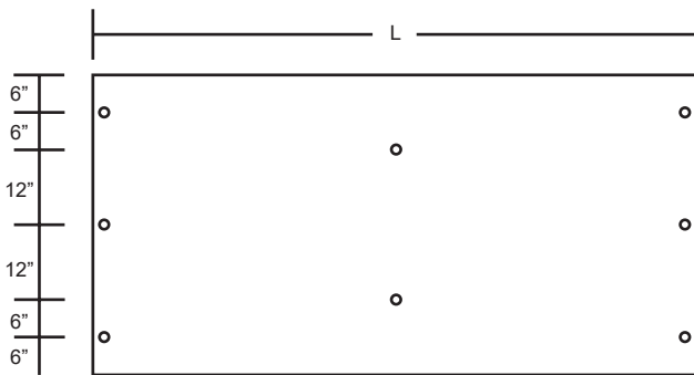
Connection patterns for two span condition
