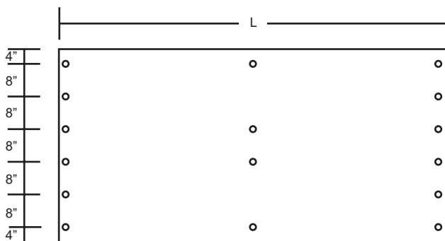
Connection patterns for two span condition
