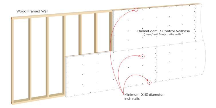
Notice: ThermaFoam R-Control insulation contains a flame retardant; however, it should be considered combustible and should not be exposed to sources of ignition. The product will ignite when exposed to open flame or welding torches.
