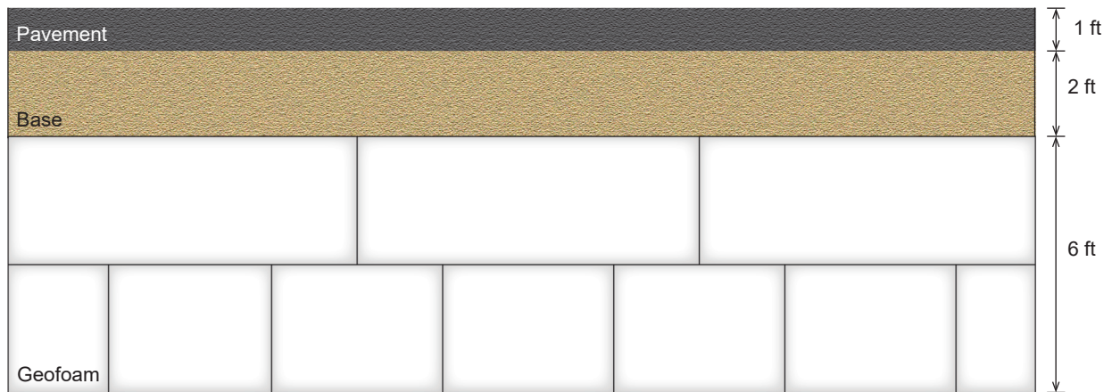
Figure 3. Calculations for dead loads
