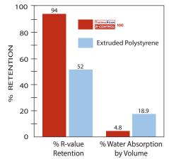
Retained thermal resistance and water absorption of insulations subjected to 15 years below grade exposure
