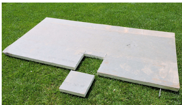
Figure 5. 17 year old polyiso sample
