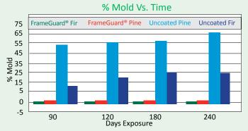
After one year and 76.3" of rainfall, there was significantly less growth of mold on corresponding samples of FrameGuard® wood. Weather-shielded samples of FrameGuard® wood had virtually no mold after the year's test.
